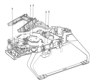
Use a 2.5 screwdriver to remove the 6 screws securing the Central Compartment Cover, and disconnect the connectors on the Central Compartment Cover and gently remove the cover and the feeder.
