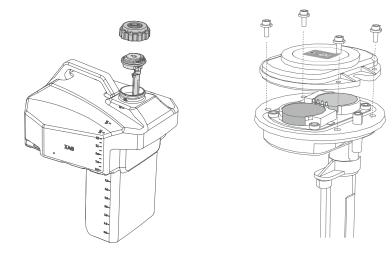
Ensure the integrity of the Waterproof rubber ring for Pump Housing and Peristaltic Pump, avoid liquid or foreign matter from entering.
