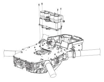
Use a 2.0 screwdriver to remove the nine (9) screws securing the Peristaltic Pump Housing
