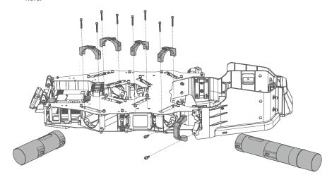
5. Disassemble the Propeller, Nozzle, MotorHousing and Motor.
