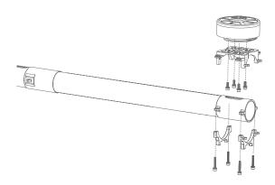
Inspect and ensure the Landing Skid, Anti-Loosening Joint, and the Suspension fixture of the Landing skid are firmly secured.
